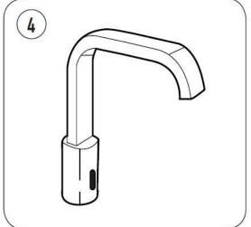
Unscrew the screw on top of the bateries box and introduce the new bateries.
